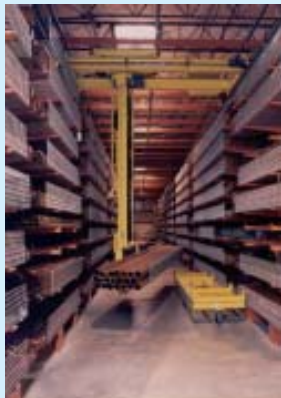
Copper Tube Storage System on Cantilever Rack
