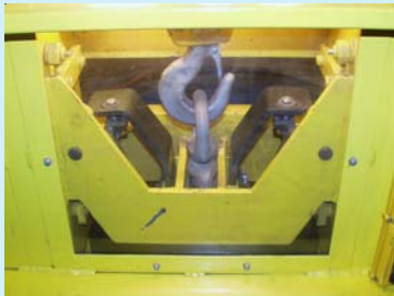
Anti-Free Fall Safety Device
