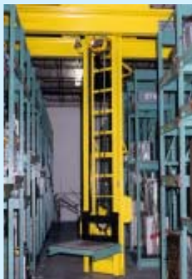
Stacker Crane Retrofit to Existing Racking System
