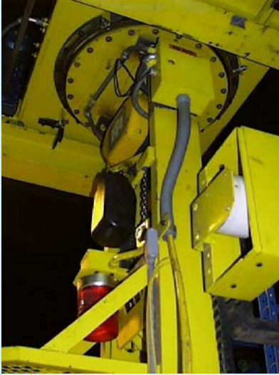
Internal Geared Slewing Bearing For Mast Rotation
