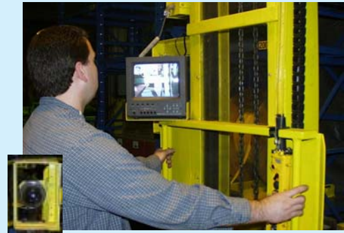
Operator's Station with Remote controlled Color Video Monitor and Adjustable Camera
