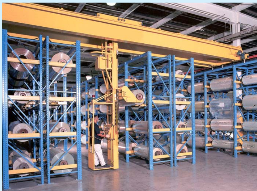
Multiple Aisle Storage System featuring One Stacker Into Multiple Bays
